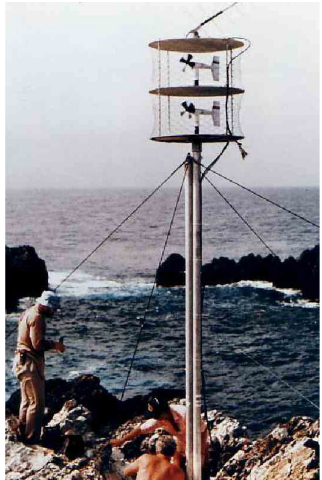
An innovative method of discouraging interference from birds was used at a station at St. Peter and St. Paul Rocks (Brazil). Photo courtesy Dr. Silvia L. Garzoli (Director of the Physical Oceanography Division of the Atlantic Oceanographic and Meteorological Laboratory of NOAA).
